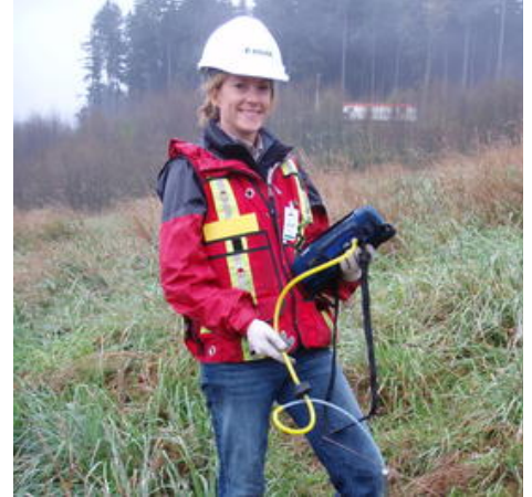
Residuals stockpiled for use on landfill closure (left). Landfill gas monitoring is conducted to determine barrier layer requirements (right).
