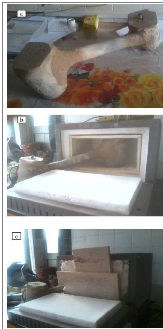
Figure 5: bench scale system for pyrometallurgical Zn recovery
