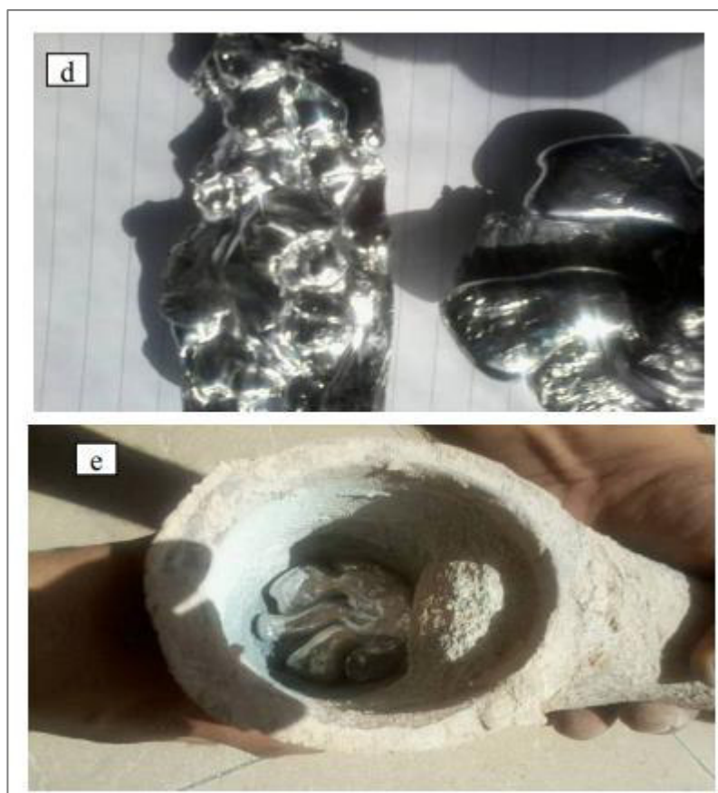
Figure 6: A photograph of the pyrometallurgical system used for Zn recovery and recovered zinc from Zn-dross
