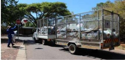
**“Separate vehicle”**: S@S is done by households /industry; kerbside collection in separate vehicles (by municipality, contractor/private sector or cooperative); The recyclables will be sorted and baled at clean MRF; residual waste transported to landfill
