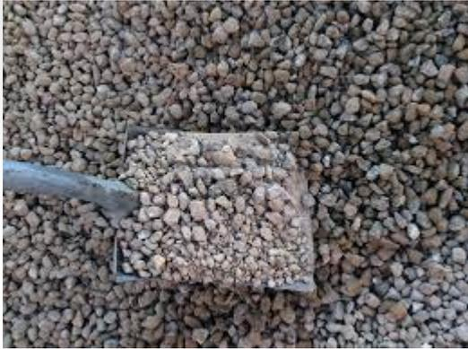
Figure 3: Sub base aggregate
