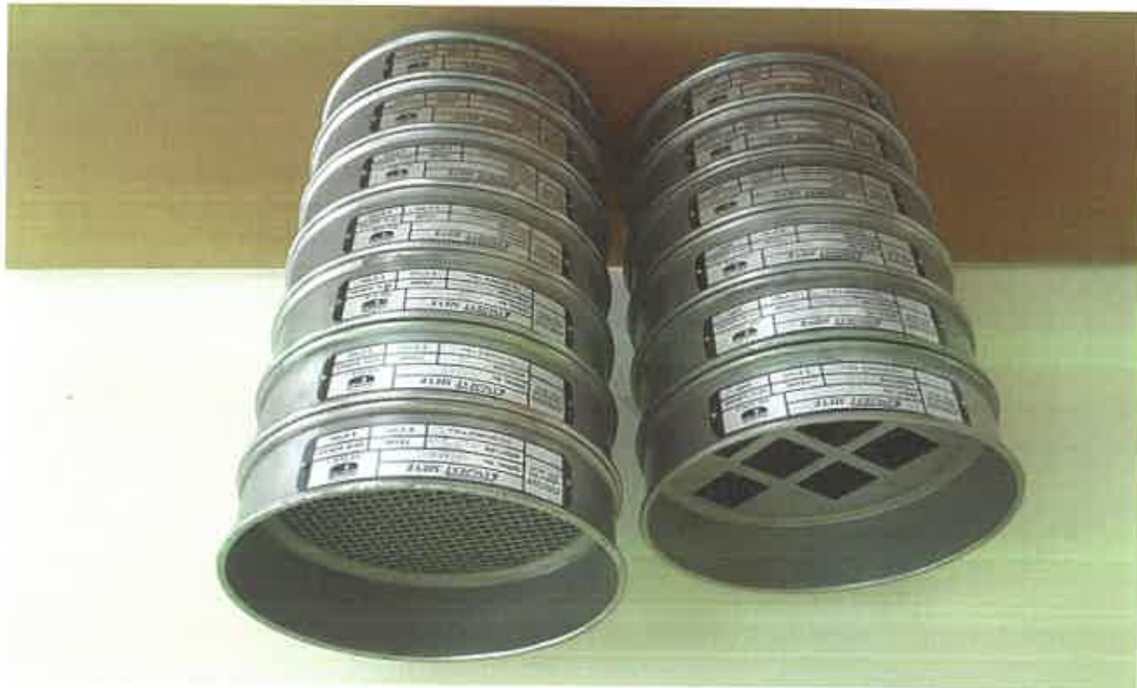
Figure 6: Two nests of sieves were used for separating the samples into coarse aggregate (see LHS nest) and fine aggregate (see RHS nest).
